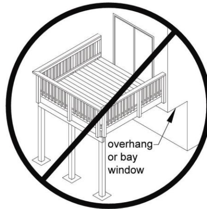
Figure 18. No Attachment to House Overhang with Ledger.
